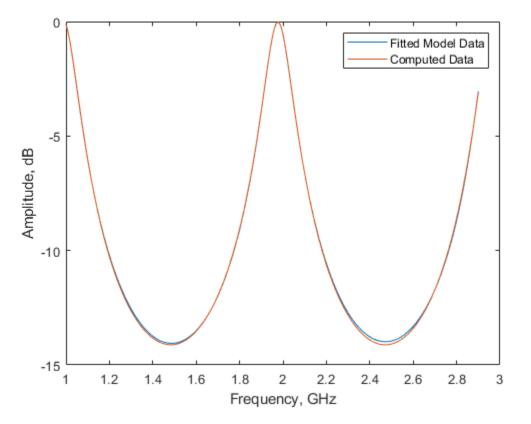
The amplitude of the model data is very close to the amplitude of the computed data. You can control the tradeoff between model accuracy and model complexity by specifying the optional tolerance argument, tol, to the rationalfit function, as described in "Export Verilog-A Model".
