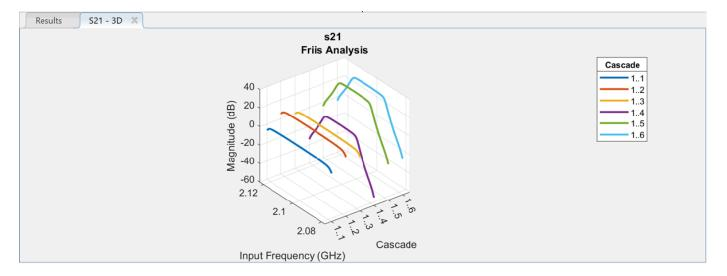
Select the **S-Parameters Plot** button. In the **S-Parameters** pane, type 6 in the **Select cascade up to stage** box. This allows you to plot Smith® chart, polar plot, magnitude, phase, real, and imaginary parts of the S-parameters of the RF System over stages. In the **XY Plot** pane, select the **S11** check box, and in the **Plot Plot** pane, select the **S21** check box. This displays the S11 and S21 in the XY plot and polar plot respectively.
