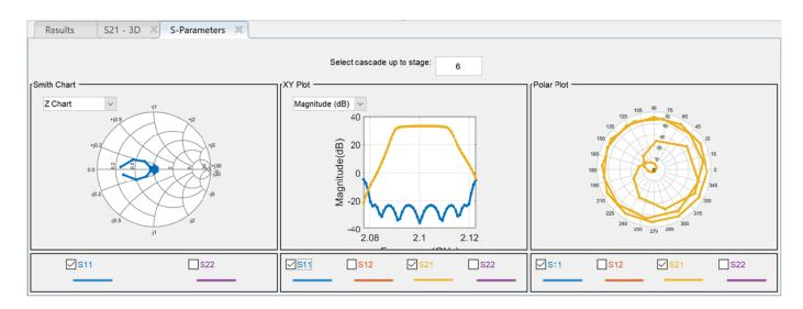
To analyze your system using the harmonic balance solver, in the **Harmonic Balance** section, select the **HB-Analyze** button. Harmonic balance results are dispayed in the **Results** pane. To compare the results, select the **Compare View** check box.
