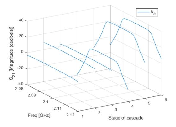
Plot the magnitude of the S21 parameter for the cascade at stage 6.
